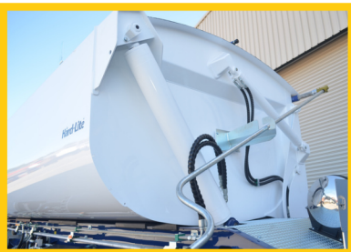
■ Formed coaming sections & complete body fabricated from Hardox.
