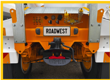
■ Fabricated tow bracket to rear with air, electrical, hydraulic couplings and coupling of your choice.
