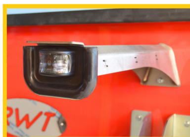
■ Hella LED lights fitted to stainless steel arms with rubber protection.
