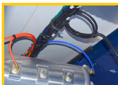
■ Wiring harness and air lines neatly secured against the chassis to reduce damage and for ease of maintenance.
