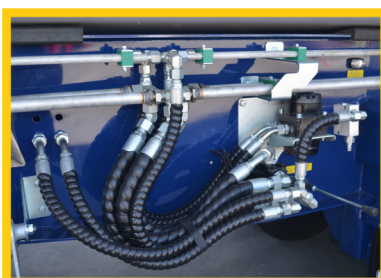
■ Stainless steel hydraulic pipes and hoses covered in spiral conduit to minimise wear, positioned in optimal location.
