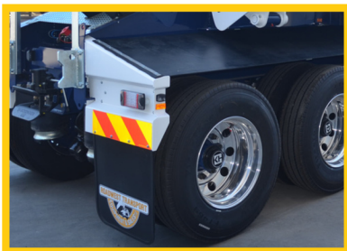
■ Durable RWT mudflaps and flexiguard to prevent mud build-up and stone chip damage to trailer.
