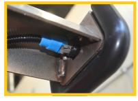
Plug and play wiring loom using double O-ring sealed Deutsch plugs.
