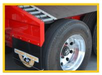
Durable RWT mudflaps and flexiguard to prevent mud build-up and stone chip damage to trailer.
