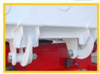
Mechanically operated door locks to ensure door fully seals.
