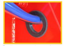
Rubber grommets to reduce wear and tear on electrical and air components.
