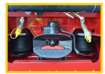
Fabricated tow bracket to rear with electrical couplings. Rubber protection as standard. Tow coupling optional.
