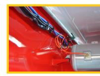
Wiring harness and air lines neatly secured against the chassis to reduce damage and for ease of maintenance.
