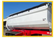
Unique pressed 'U' shaped body for increased stability whilst tipping, eliminating product 'hang-up' and improves flow of product for quick discharge.
