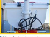
50 tonne five stage external trunnion mounted hoist.
